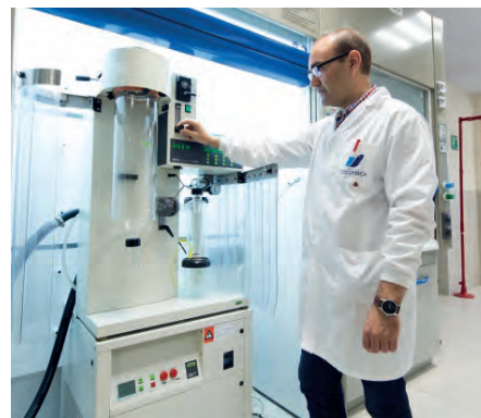
Spray dryer system
